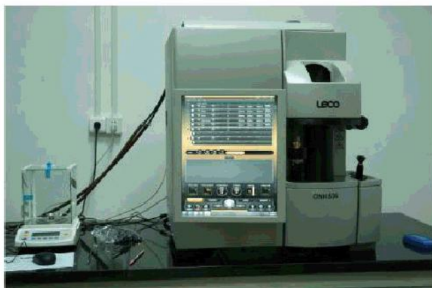
氧氮氢分析仪 Oxygen Nitrogen Hydrogen Analyzer 分析钕铁硼磁铁里的氧氮氢的含量。 Analysis the content of Oxygen Nitrogen of NdFeB magnet.
