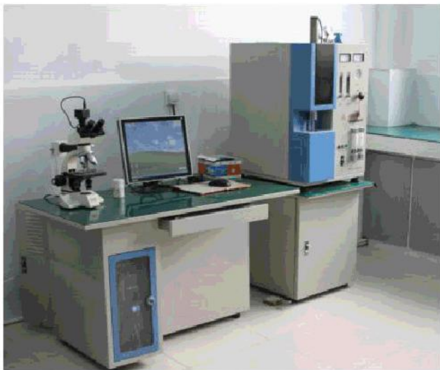
碳硫分析仪 Carbon Sulfur Analyzer 分析稀土里的碳硫含量。 Analysis the content of Carbon and Sulfur in Rare Earth.
